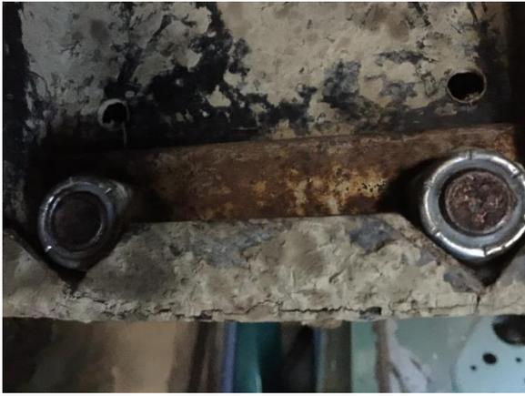
The chief scrutineer at the National Rally advised me to fit a spreader plate on the rear tow hitch on the inside of the rear cross member. I have now fitted one, the plate is 6mm thick. The vehicle reg is YVF 984A.
